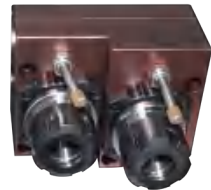
Two power heads on both sides of the detachable end
